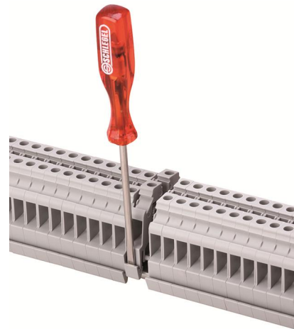
10b. Snap fitting of pre-assembled terminal blocks Important: Once the terminals are mounted onto the rail, the snap-fit terminal feet are relieved from stress preventing the plastics from material fatigue.
