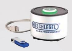
The programming station belonging to the management software consists of a desktop housing and a reading/writing unit with USB connection. Together with the management software the transponders can be programmed simple and easy.
